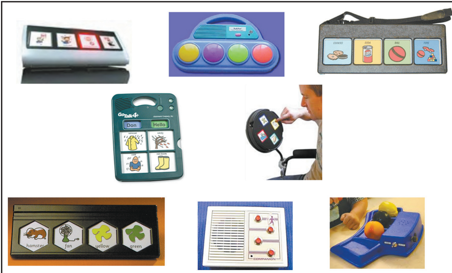
Figure 7. At least 7 companies provide a wide variety of options in four-message devices. Top Row: AbleNet's FLASH, Frame Technology's Talkpad, AMDi's Partner/Four. Middle Row: Attainment's GoTalk 4+, Enabling Devices' Round Cheap Talk 4. Bottom Row: Inclusive TLC's 4Talk4, Lumin-aud's Companion 401 Communicator, Enabling Devices' Take N' Talk.
