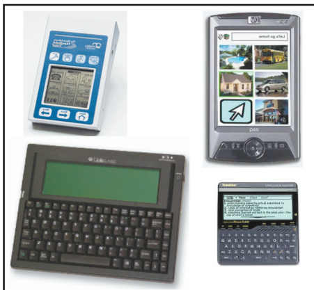
Figure 14. On the top left is the Hand Held Voice by Ability Research and on the right is the Cyrano by OneWrite. On the bottom left is the Link Classic by Assistive Technology Inc. and on the right is the Speaking Language Master by Franklin Electronic Publishers. All of these devices, usually considered high tech, meet the cost criteria for lite technology as defined for this survey.
