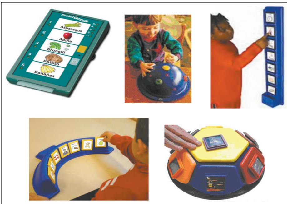
Figure 8. A limited number of options with 5 to 7 messages. Upper left: Attainment's Pocket GoTalk. Remaining devices are from Enabling Devices: Talking Bubble, Take N' Talk Go! Board, Take N' Talk Tabletop, Carousel Communicator.
